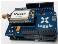
Figure 5 - Arduino fitted to Corella Arduino Shield
