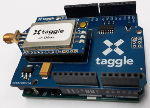
Figure 6 - Arduino fitted to Corella Arduino Shield
