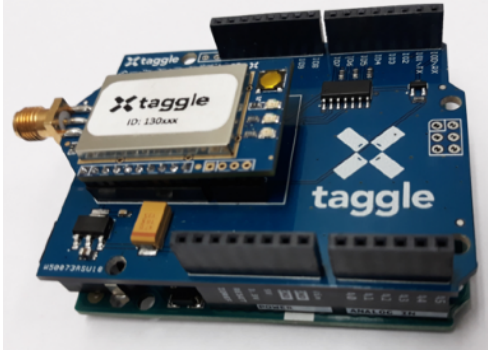
Figure 6 - Arduino fitted to Corella Arduino Shield
